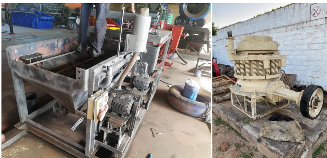
Figure 3 & 4 – DMS unit undergoing modifications and refurbishment in South Africa and Cone Crusher refurbished in South Africa, factory acceptance tested in Zimbabwe
